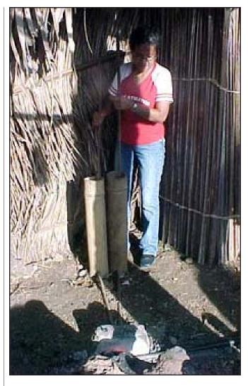
While the metal is all brought in from outside, Bukoli residents are able to shape it with this simple forge. The bellows are two huge bamboo stalks with wooden plungers and an intricate shutter valve at the base. Wood is burned between the stones, and a rod whose tip is in the fire lies to the right. Tips for digging sticks and machete blades are made on this forge.
