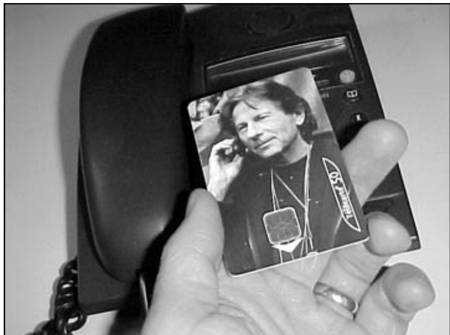
This picture is not about Roman Polanski but about smartcards. The microchip that makes them “smart” is the small rectangle at the bottom.
