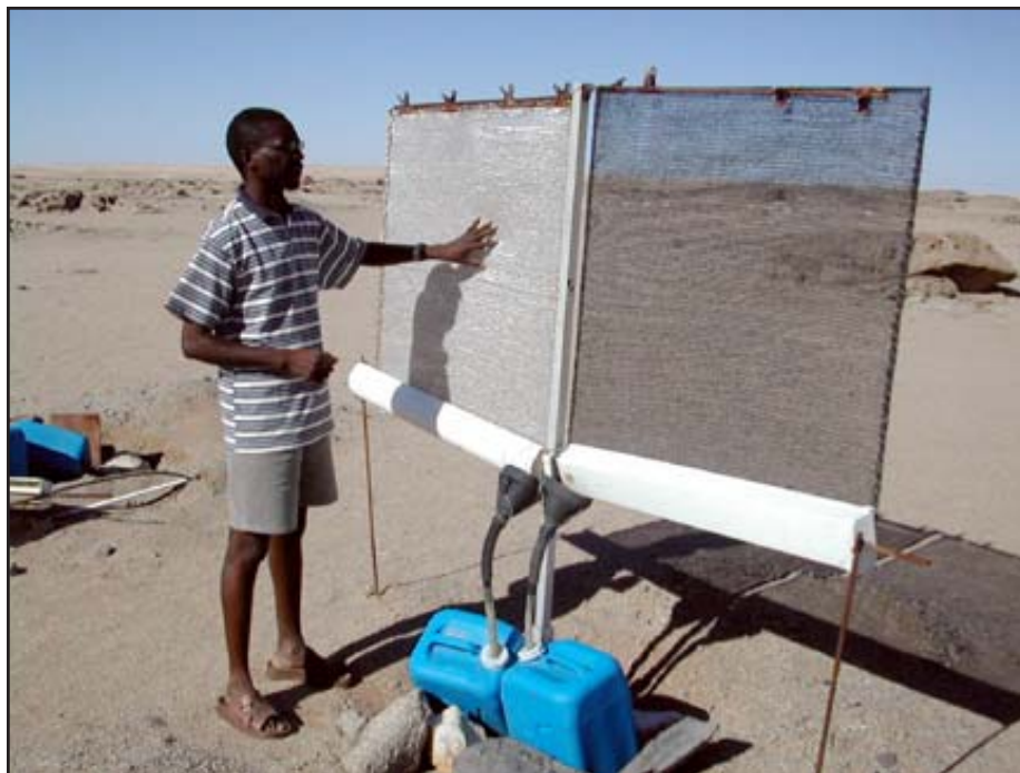
Vilho 'Snake' Mtuleni: "We have good, affordable material, and technology. A weak point remains how to keep these [collectors] clean and upright when a sudden sandstorm comes along."
