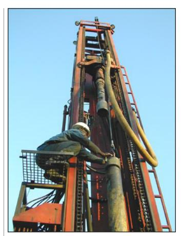
**Avast Up Thar Matey:** A Prinsloo drilling-crew member leans out of the crow's nest, uncouples the baling clamp and prepares to screw in a drill-pipe segment.
