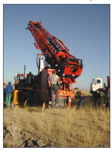
**Erect, Set, Drill:** Lawrence Prinsloo at control panels 'hoists the mast' on his mobile drilling rig in the prep stage of punching a borehole in the earth
