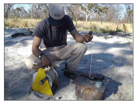
**Why Dry**? Brickhill uses a Piezometer test to compare moisture level in a nearby borehole that did not yield enough water at its depth.
