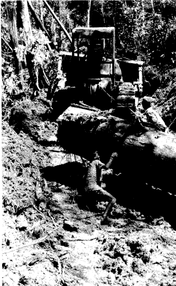
Looping a steel cable around a log to pull it through a turn in the skid trail
