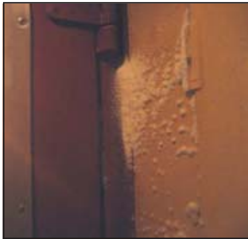
A raging snowstorm invades the unheated space between train cars. Photo: Bert de Muynck
