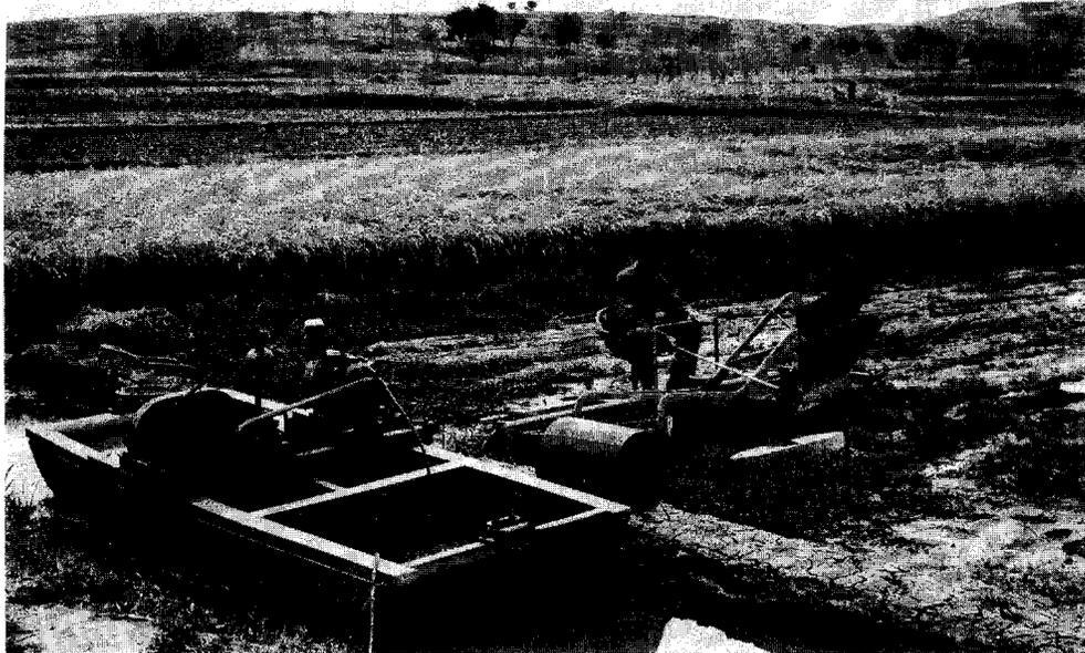
The cable towed plough. Demonstrated outside the Agricultural Mechanization Research Institute, Nanking. The winch on this boat is powered by an electric engine.
