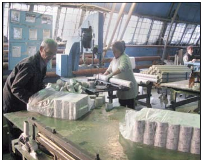
(Above) Inside Vtorma's factory, above the sheet of recycled paper, is a poster saying, "One who's friends with vodka is not needed at work" (it rhymes in Russian). (Below) This is how a long roll of recycled paper transforms into a ubiquitous toilet roll.
