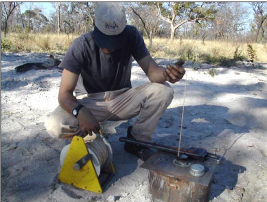
**Why Dry?** Brickhill uses a Piezometer test to compare moisture level in a nearby borehole that did not yield enough water at its depth.
